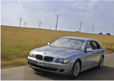
Figure 10. Mauvais: BMW Hydrogen 7. 245 kWh aux 100 km. Photo: BMW.
